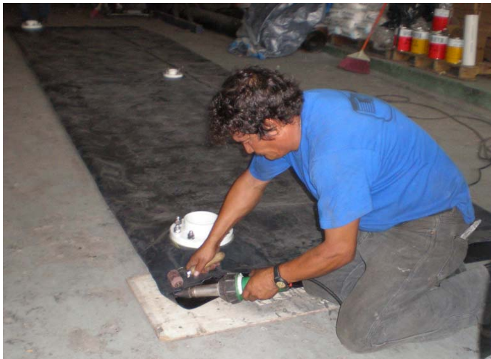
Figure 25. Fabrication of an early improved biodigester. A heat gun and roller is used to seal the plastic. Heavy and expensive PVC tube adaptors can be seen for the inlet and outlets connections.
