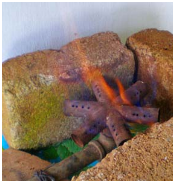
Figure 17. A simple star burner burning biogas. It is difficult to photograph biogas flames as they are generally clear or light blue.
