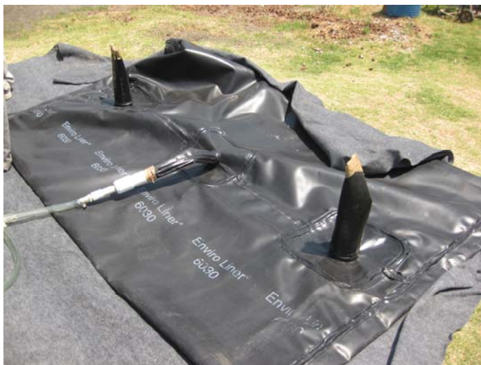
Figure 23. A recently (April 2009) built improved digester with the sleeves of the system that will connect to the PVC inlets and outlets visible. This digester is not installed and has just been unwrapped onsite for inspection before the installation at GIRA.
