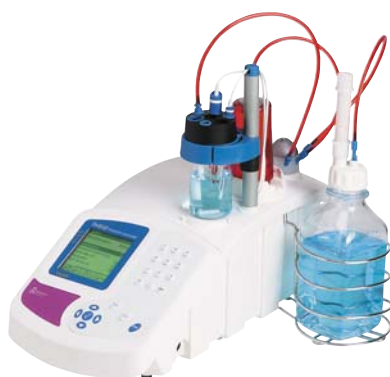
Automatic titrator for the volumetric determination of organic acids
