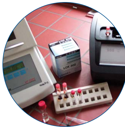
Fig. 6: Photometric measuring station: HT 2005 thermostat, cuvette test, DR 2800 photometer
