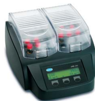
Dry thermostat for all standard digestions
