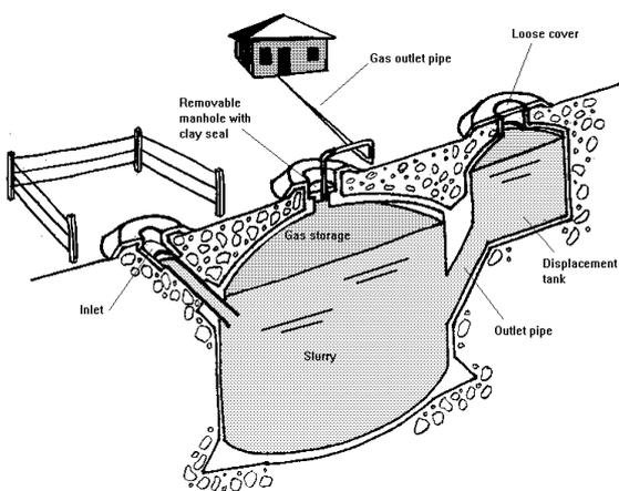
Figure 1: Fixed dome digester
