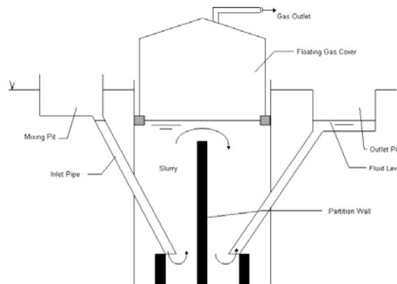
Figure 2: Floating cover digester
