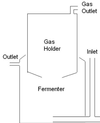
Figure 3: Compact biogas digester
