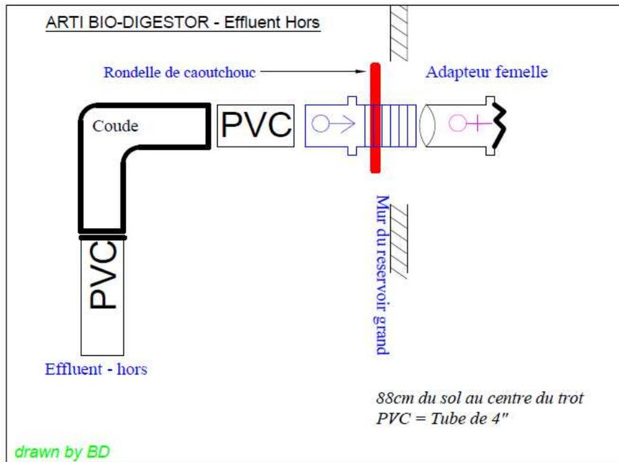
The female fitting used on the inside of the tank for the residue outlet must be cut short with a hacksaw. If it is not cut there will not be enough space for the gas holder to fit inside the fermentation tank.
