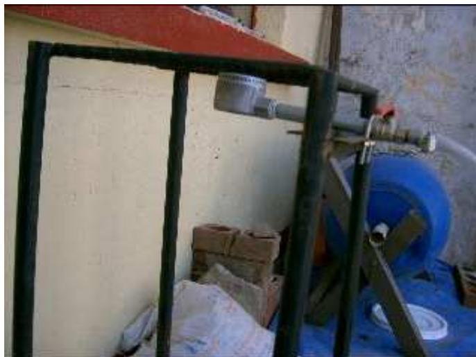
A stand for the gas burner can be welded from iron bar (1.5cm Ø + 2.5cm Ø tubular iron for the legs.) The fittings needed to attach the gas hose to the burner are as follows:
