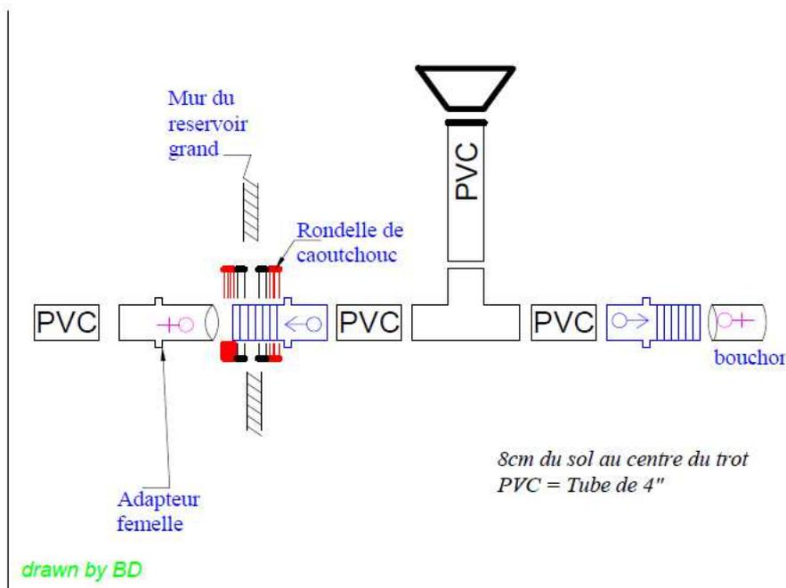
Tank interior is on the left. There are two rubber washers and a thicker washer (black) on each side of the tank.
