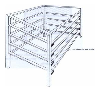
Fig. III A *brooder box* measures 2' x 4.5 x l' and can accommodate 200 chicks. A 50 watts bulb is needed to give heat to the chicks
