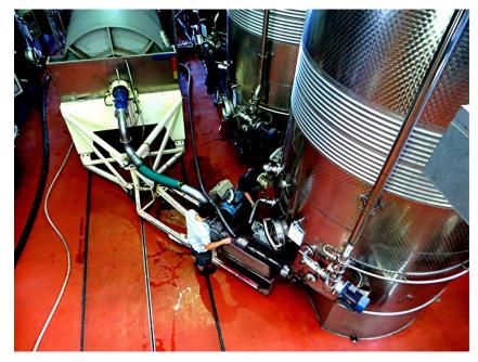
with grape juice and red grape skins that had been stored together. They were pumping the mixture into the cylindrical machine on the left in the picture. Inside that machine the juice skins mixture was processed through a sieve that held back the skins and let the red grape juice pass through. The red grape juice was then prepared for the process of making red wine.
