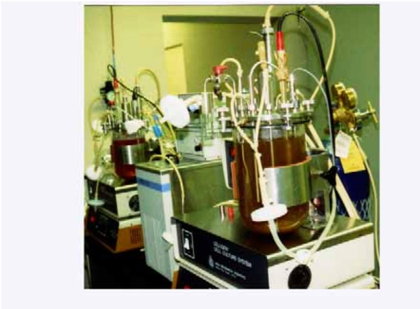
**Plate 3. A model of a programmed cell culture system with glass jars (Courtesy Jun Mitsuhashi)**
