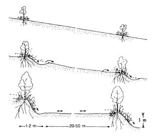
*Figure 11: Hedgerows leading to terrace formation Source: Agrodok 13: Water harvesting and soil moisture retention*
