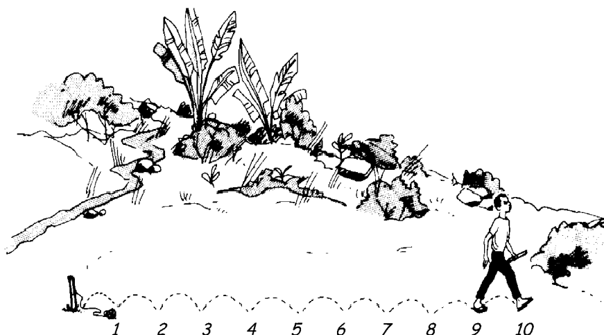
Figure 28: Staking out the pond (Murnyak and Murnyak, 1990).
