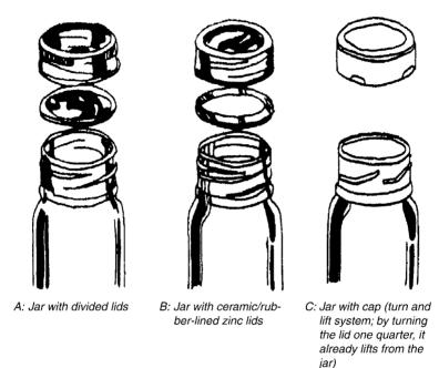
Figure 2: Glass jars with different sealing mechanisms
