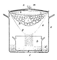
a: sterilizer or washkettle b: enamelled pan or stoneware dish, collecting the juice c: heat source d: water for evaporation e: steam f: supporting rack or plate g finely woven cloth as a juice filter h: coursely woven cloth i: fruit k: condensation m: muslin cloth tied around the lid n: cork in the thermometer hole
