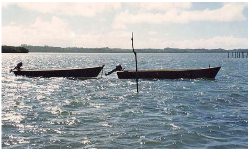
Figure 4. Eighteen-foot punts with 15 hp outboard engines provided to farmers.
