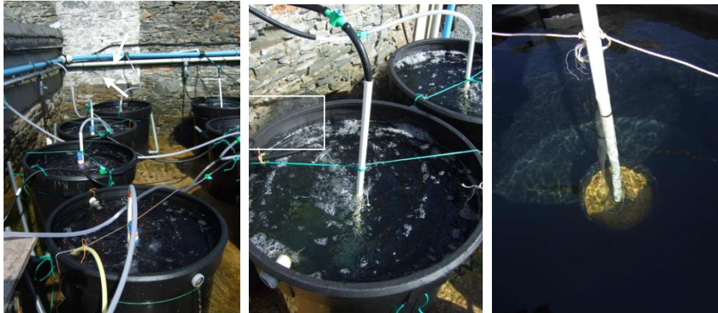
Fig. 8.2. Experimental 200-L tanks for Palmaria cultivation. Left: Overview of set-up. Arrows indicate the main supply pipes for air (blue) and seawater (grey). Middle: Seawater is supplied through a tube (2 cm diameter; white box) and air by a central pipe. Right: Aeration pipe with weight at the bottom made by filling a flowerpot with concrete.
