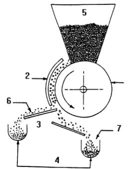
Figure 3 : Separation of pulp and beans
