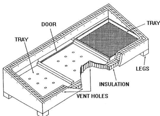
The drier should be filled with coffee as early in the day as possible so that all possible sunlight hours are used. The coffee should be stirred regularly so that a uniform colouration is formed. At night, the crop should be transferred to a cool dry room to prevent moisture condensing on the coffee.
