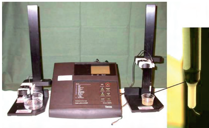
Figure 3: Photograph of the microtouch instrument, to the right, an enlarged picture of iridium touch microelectrode with a diameter of 0.1mm.
