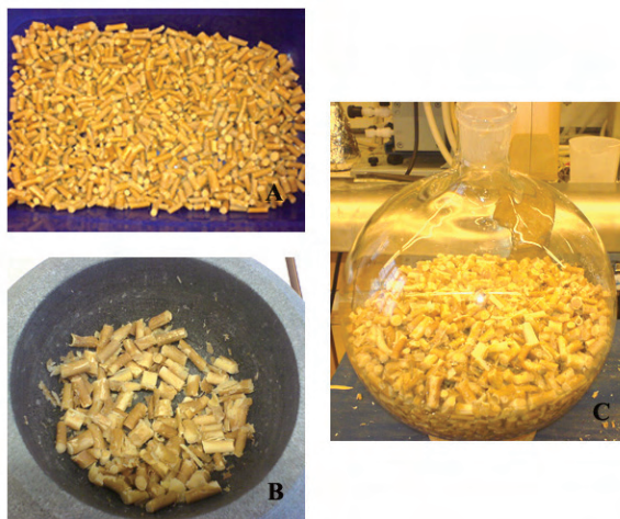
Figure 13: A) Miswak roots cut into small pieces. B) Miswak root smashed with a stone mill. C) Miswak root pieces in round bottomed flask.
