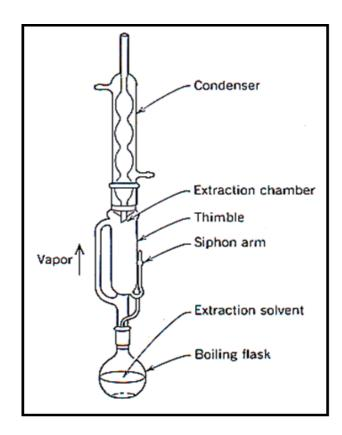
Figure 3. Experimental setup soxhelet extractor apparatus
