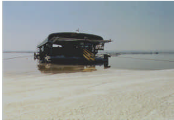
Figure 5: Dead Sea Works salt harvester on evaporation pond
