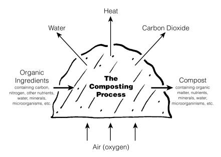
Figure 2. Basics of the composting process
