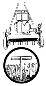
Figure 12. Power rakes and vertical mowers are designed for thatch removal. These machines have blades, knives or tines mounted on a horizontal reel or shaft which revolve in a plane that is vertical to the ground.
