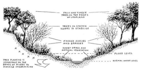
Figure 8.17 Stream-bank protection
