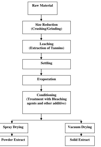
**Figure 1:** Process Block Diagram for the Manufacture of Vegetable Tannin Extracts.
