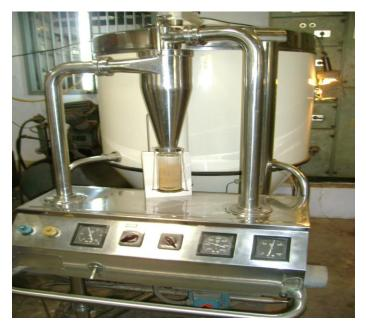
Figure 3: Co-current spray drier apparatus
