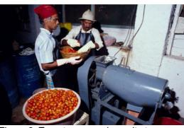
Figure 3: Tomato processing unit at Walewela, Sri Lanka. Putting tomatoes in the pulper. Photo: Practical Action / Zul.
