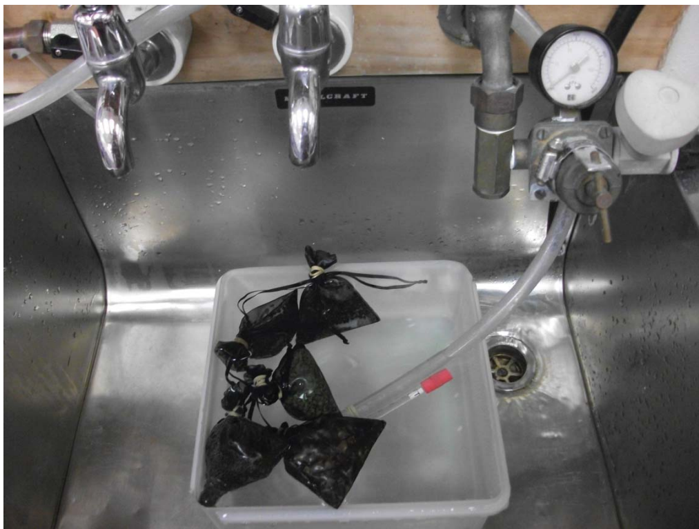
Figure 6. Washing fruits in organza bags with running water. Thermometer for monitoring temperature is attached to the plastic tubing.
