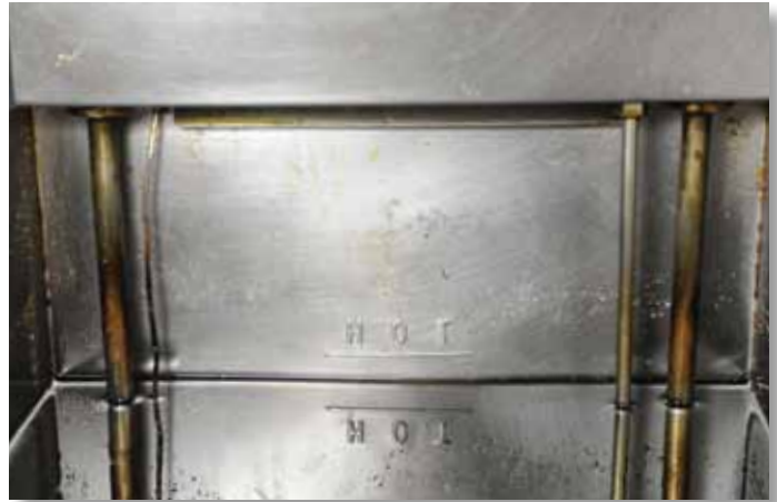
Polymer buildup on fryers after cooking French fries for 13 8-hr shifts. The equipment settings and all other conditions were the same for both fryers, except that the fryer on the left contained commodity soybean oil, and the fryer on the right contained Pioneer's high-oleic soybean oil.
