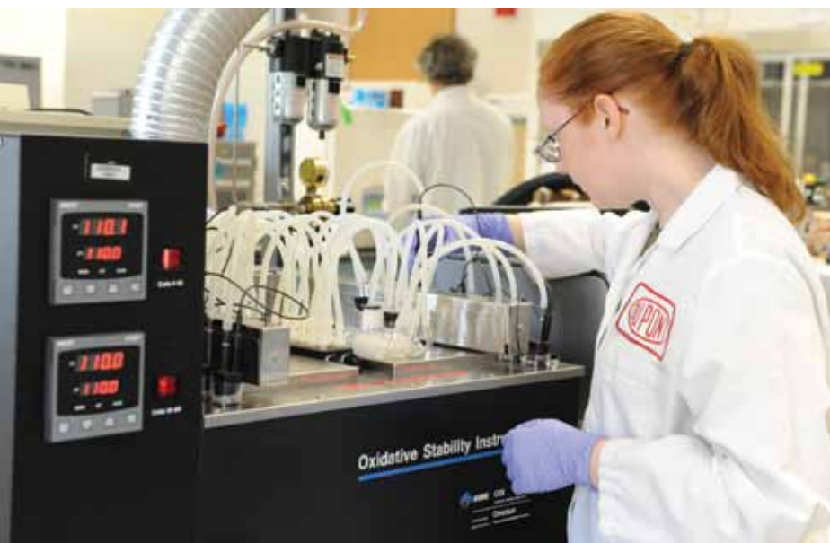
DuPont technician sets up the Oxidative Stability Instrument for testing Pioneer's high-oleic soybean oil.
