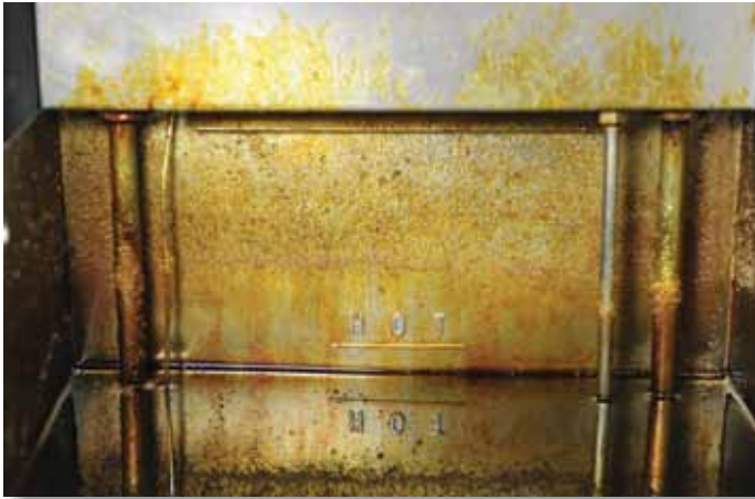
Polymer buildup on fryers after cooking French fries for 13 8-hr shifts. The equipment settings and all other conditions were the same for both fryers, except that the fryer on the left contained commodity soybean oil, and the fryer on the right contained Pioneer's high-oleic soybean oil.
