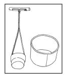
Figure 7. Core sampler and screen bucket.
