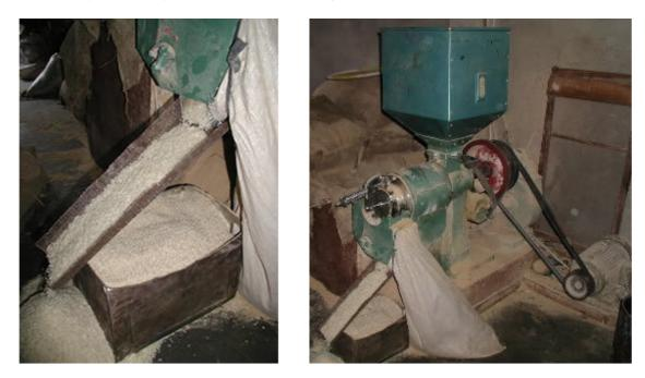
Installing a 1.4 mm round screen on the outlet of a horizontal friction whitener (as shown), will reduce the amount of small brokens, chips, and germs from the milled rice. The material that falls through the screen can be used to make rice flour.
