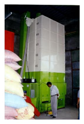
Medium-sized grain dryers such as this recirculating batch dryer are now a common sight throughout Asia. In general, mechanically dried grain will produce better quality of rice. Grain recirculation allows for uniformly dried grain, and automatic drying air temperature control will reduce overheating or overdrying.
