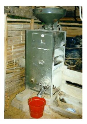
An example of a rubber roll mill is the compact 2-stage rice mill which has 0.5 to 1 ton per hour paddy input. A typical compact rice mill consists of a 6-inch diameter x 6-inch wide rubber roller husker, and a friction whitener. The friction whitener has a very similar design configuration as the Engleberg except that is has no husking knife. The milling performance of the compact rice mill is superior to the single pass Engleberg huller. Milling recoveries are normally above 60%.
