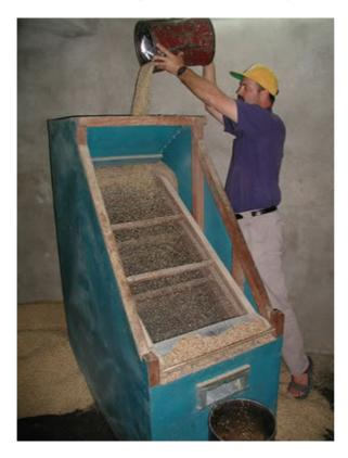
A very simple separator with no moving parts is the screen separator, which can be seen in smaller commercials mills located near rural markets. Brown rice/paddy will move through a number of screens that are set at 31-35° angle. The rough rice moves down the top screen, a mixture of rough rice and brown rice moves down the middle screen and finishing screen, and brown rice will accumulate underneath the finishing screen. Suggested screen sizes are represented in the following table.
