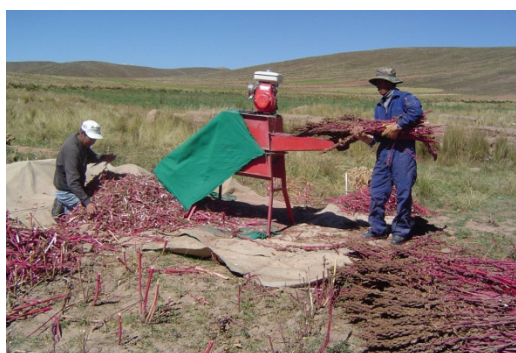
Photo 7. Threshing Method: Mechanical threshing – Central Altiplano
