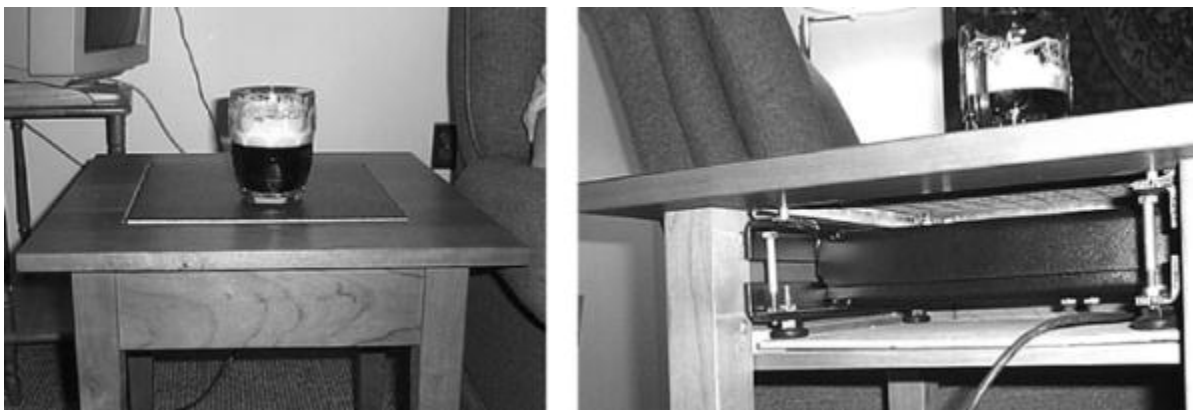
Fig. 1. The custom-designed end table with ceramic tile top is shown with a mug of beer in place (left). The scale is hidden under the ceramic tile top and serves as a base for the scale (right). This view shows that the digital scale is hidden inside the table. The view is from behind the table that normally abuts the wall and so is not typically seen by the participants.
