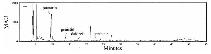
Fig. 1-HPLC profile of Pueraria tuber showing puerarin, genistin, daidzein and genistein
