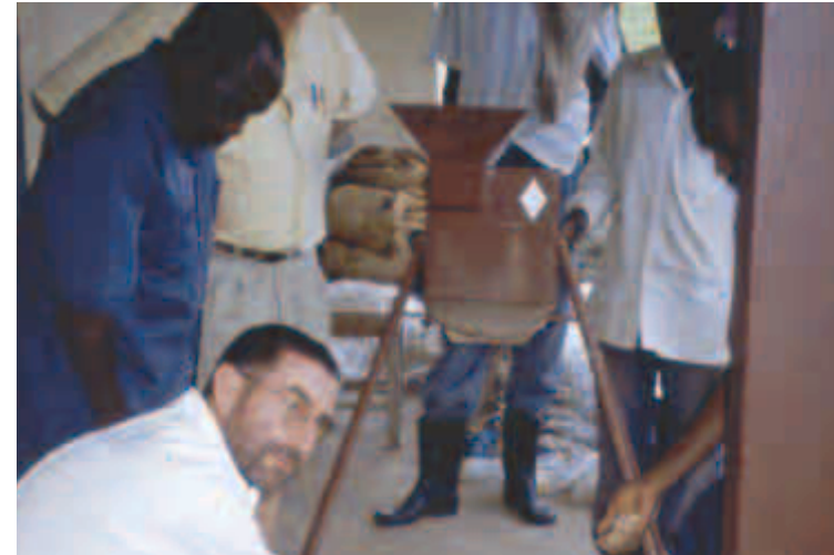
Mechanical shellers are labour-saving and the rotary design (shown here) produces very little cracking of the seed
