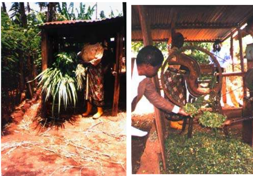
Figure 19. (left) Purity feeds Napier grass/forage legume mixture into the motorized chaff cutter while (right) the author inspects the finely chopped forage material which is ready for use
