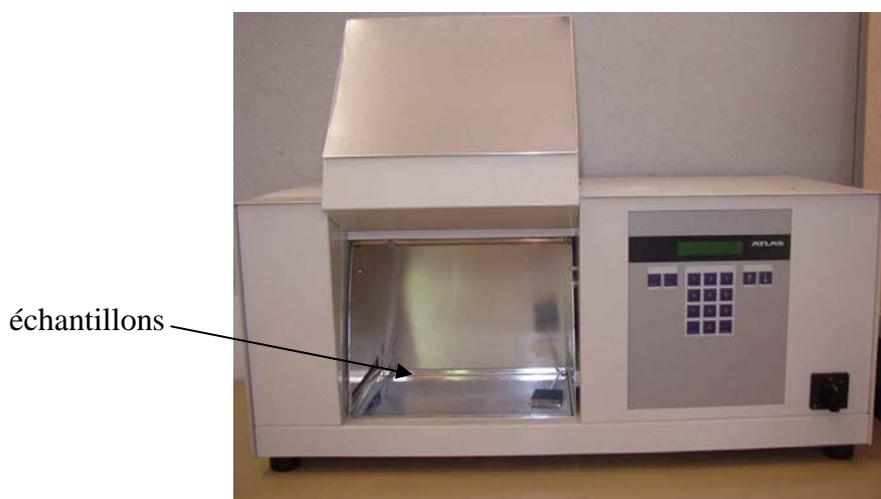
*Figure 12. Appareil SUNTEST (CPS+, Atlas).*
