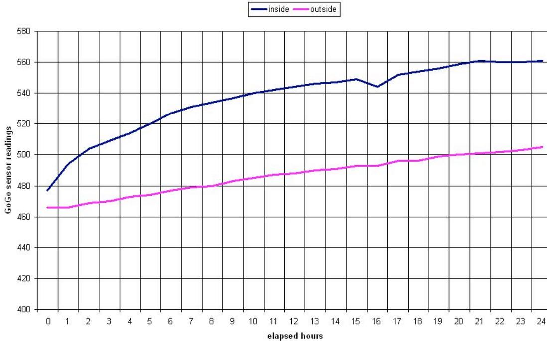
During the 24 hours we collected data it became a bit cooler both inside the pot and outside. You can see that both sensor readings increased, meaning lower temperature, during that period. During the entire time it was cooler inside the pot than outside. But, the difference increased in the first few hours. It takes a while for the Pot-in-Pot to cool down.
