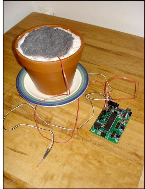
The GoGo Board does not record actual temperature. Rather, it reports a value between 0 and 1023 for each sensor reading. A reading of 0 indicates a closed circuit, such as you would get if you used a switch for a sensor and put the switch in the “on” or closed position. A reading of 1023 indicates an open circuit, such as you would get with a switch in the “off” or open position. If there is no sensor connected to a given port on the GoGo Board, the reading will be 1023.
