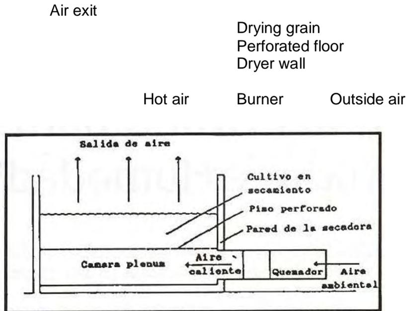
Figure 1. Plan for a batch dryer (FAO 1985)
