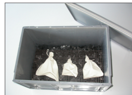
Above: "Box-dryer" - plastic box with seed collections, placed above dried charcoal, on a plastic mesh
