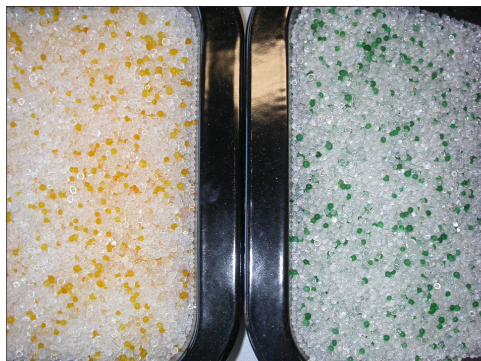
Above: Methyl violet indicating silica gel beads mixed with clear silica gel, showing dry (orange) and wet (green) status
