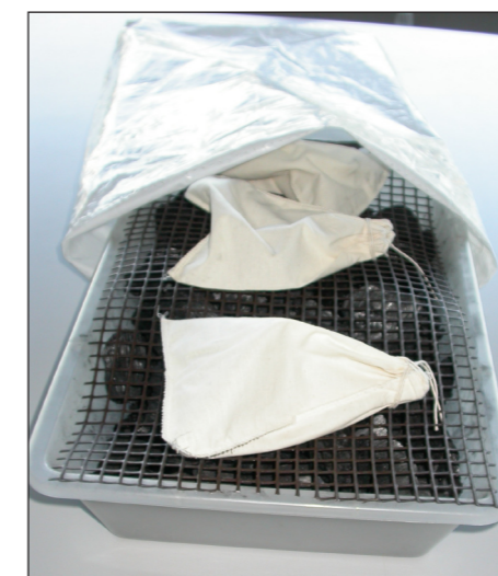
Above: "Box-dryer" - plastic box with seed collections, placed above dried charcoal, on a plastic mesh
