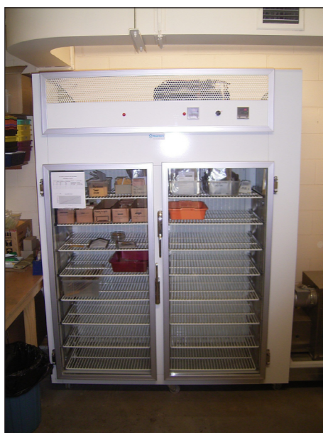
Left: Bespoke drying cabinet with a dehumidification unit, at Victoria Royal Botanic Gardens, Australia
