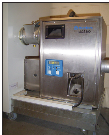
Below: Dehumidification unit attached to a drying cabinet for small-scale drying
