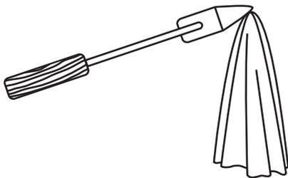
Rub the face of the hot iron in a shallow metal dish. If you are using resin then also add a little fine sand. Ammonium chloride is more corrosive than resin. It will cause the copper in the irons to deteriorate faster. Avoid breathing the vapours.
