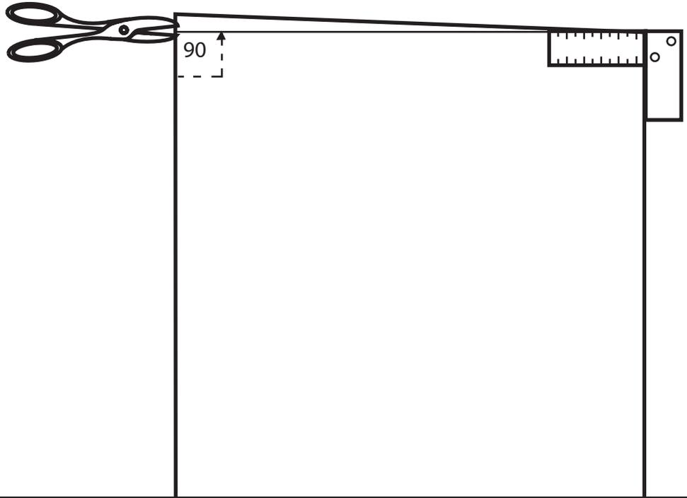
Using the measurement tools or patterns, mark the pieces for the body, openings and covers of the silo. Refer to the pages that show plans for the silo you want to build. Before starting to cut, be sure to write on each piece so you know which is which.
