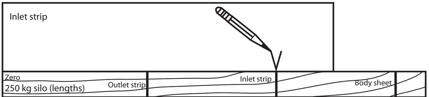
Using a story stick to mark the length of the inlet strip.
