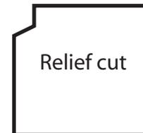
A metal pattern for marking the relief cut at each corner of the body sheets
