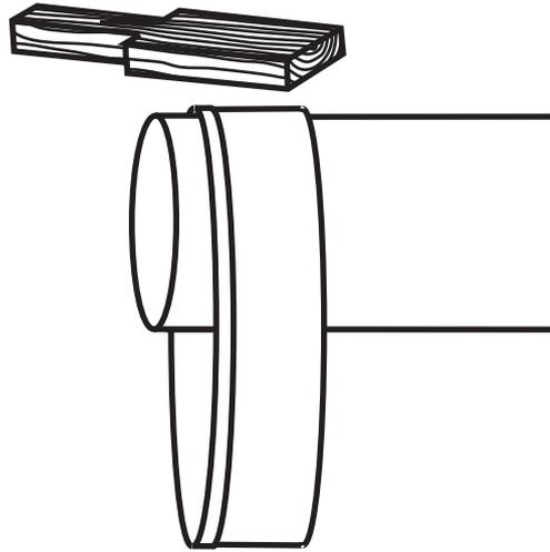
Use the flange method to join the top of the cover to the collar. Use the 8 mm bending tool.
