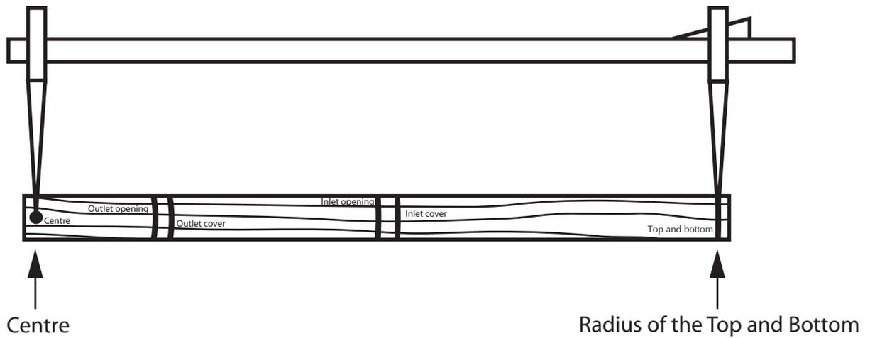
When the measurement is set, use the compass as shown in the illustration to find where to place the centre point of the circle.
