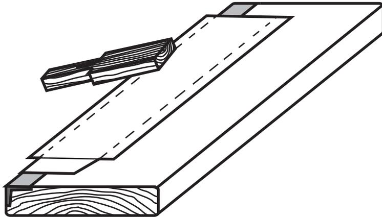
Use the hammer to close the fold but use the spacer for the last 3 cm on the end away from the tab.
