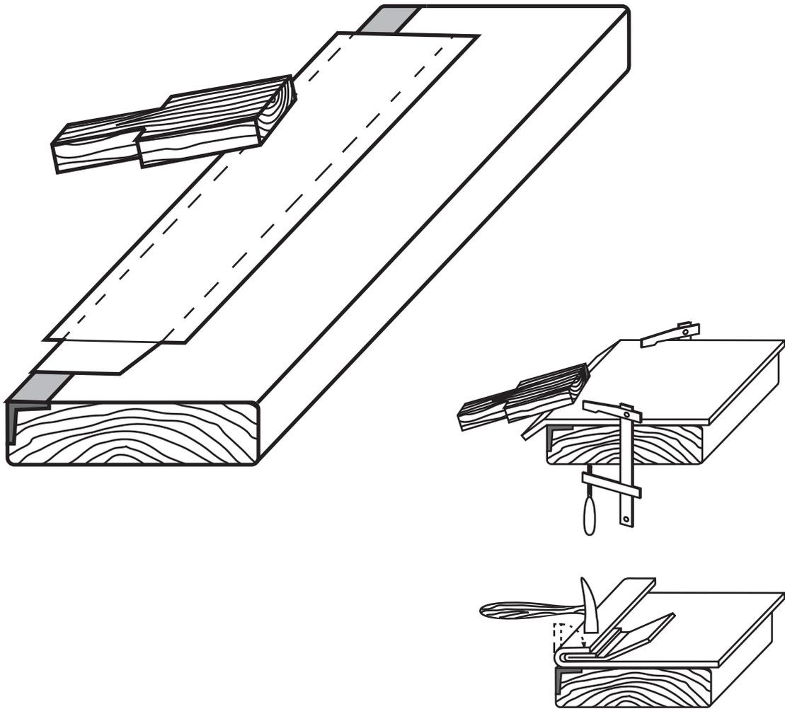
Use the hammer to completely close the fold but use the spacer for the last 3 cm on the end away from the tab.
