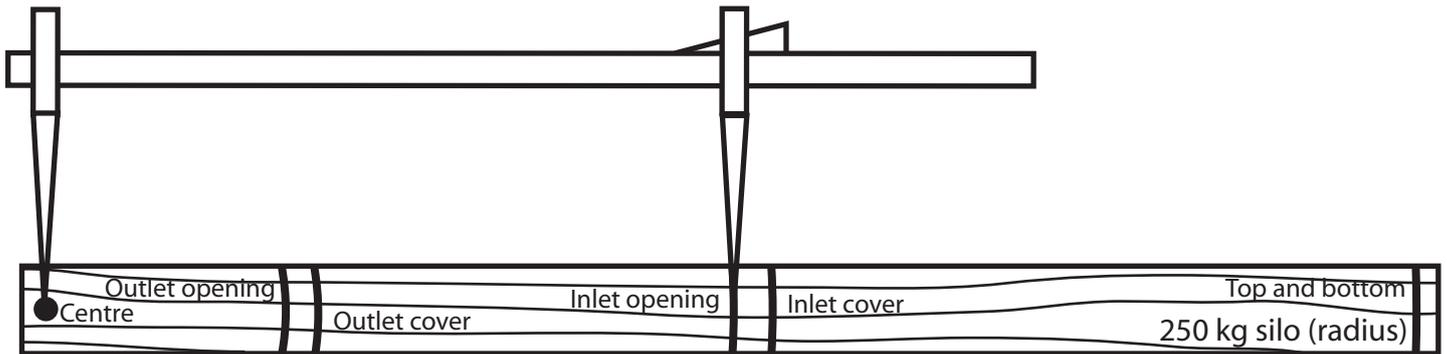
Using a story stick to set the compass for marking the hole for the inlet opening.
