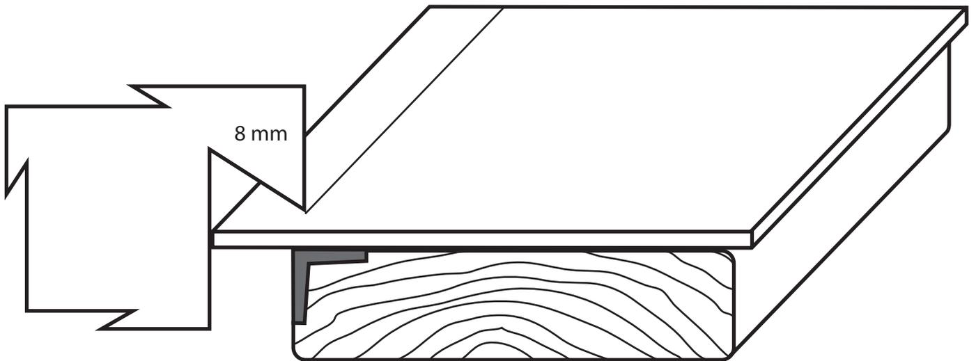
Use the wooden mallet and the edge of the bench with the angle iron to begin the fold.
