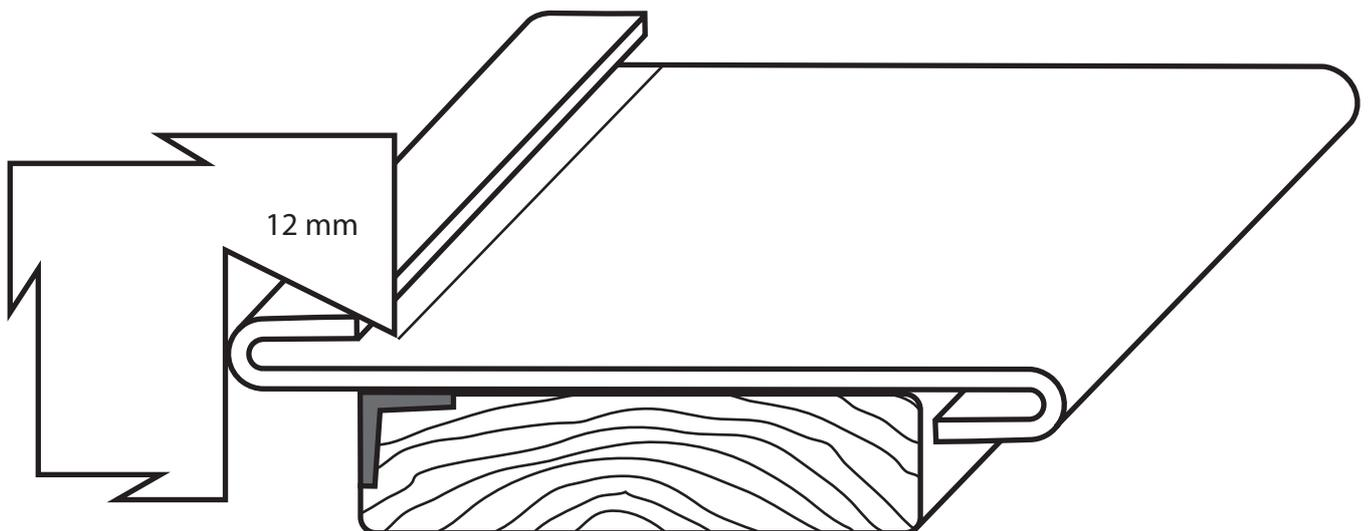
Use the spacer and the wooden mallet. Bend the edge to about 20 degrees on the bench. The edge must be bent away from the side with the fold.
