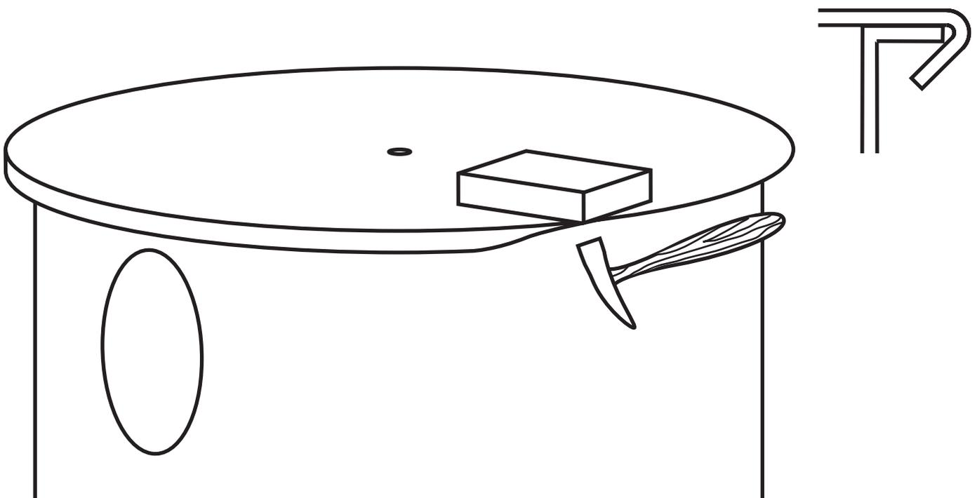
*Building the Silo* Joining the Bottom to the Body
