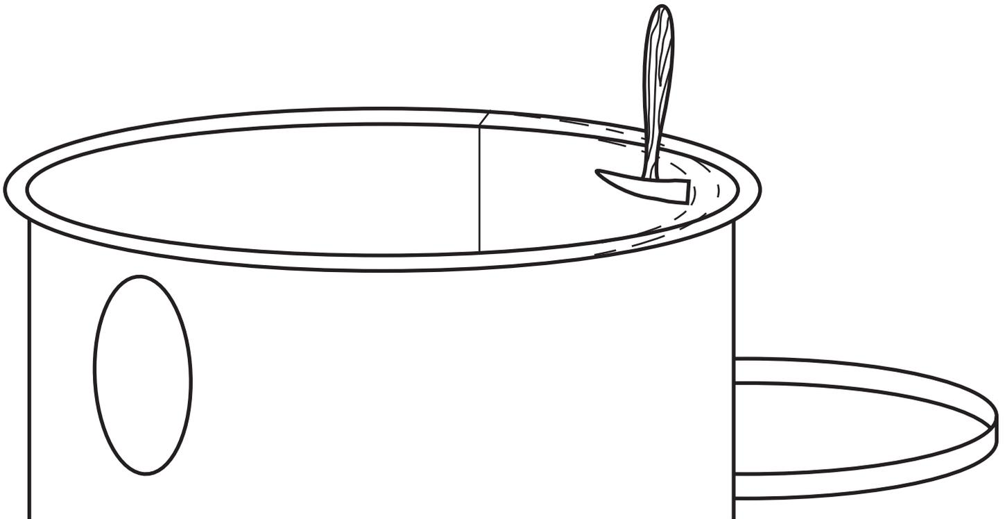
When the body of the silo fits the bottom you can start to join them together. Use the counterblow over the spot that you are hitting with the hammer as you work around the body of the silo. First, pound the flange to about 45 degrees.
