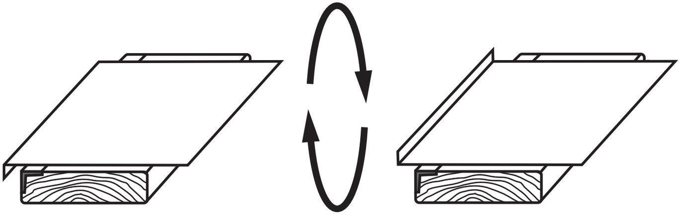
Use the spacer while you close the fold along the entire edge. At this point, the fold should be uniform and even.
