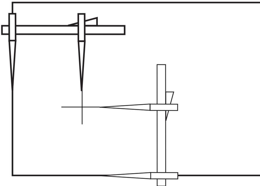
When the measurement is set, use the compass as shown in the illustration to find where to place the centre point of the circle. Don't scratch too hard or you will damage the galvanisation.
