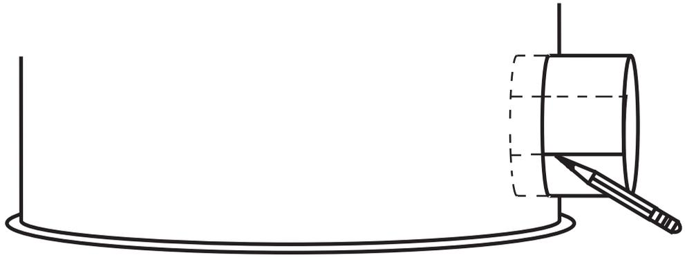
Hold the edge of the counterbore tightly against the inside of the body of the silo. The hammer blows should make a solid sound as you pound the teeth against the body.
