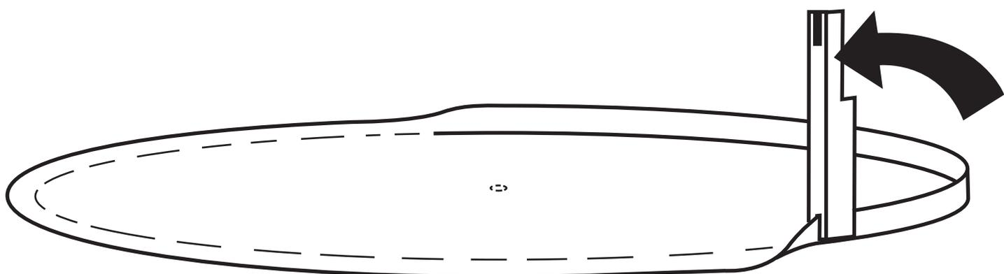
Put the bottom piece, flange down, over the body of the silo to see if they are the same shape.
