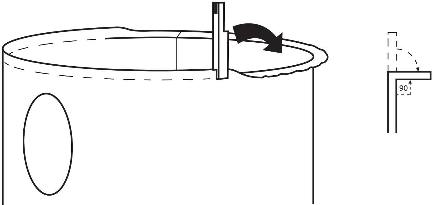
After using the bending tool, the flange will be wavy and uneven. Go around the edge carefully with the hammer and the counterblow to smooth out the flange. Stop when the flange is flat and even.
