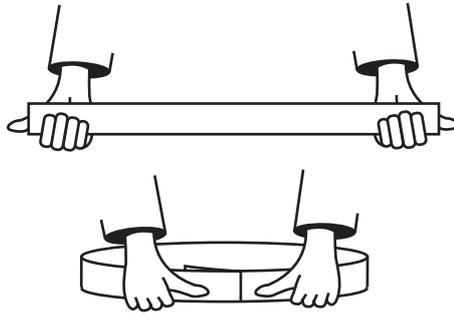
Place the strip in the hole in the top piece. Make sure that the long edges are lined up evenly. Make a mark where the end of the strip overlaps itself but don't cut it yet.
