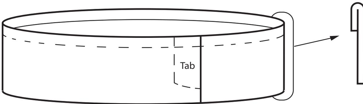
The folded edge must be pounded closed where it overlaps the tab.
