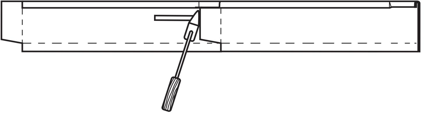
Bend the strip into a circle with the folded edge on the inside. Carefully align the measurement marks. The tab goes on the inside of the circle. The top edge of the tab fits under the folded edge of the strip.
