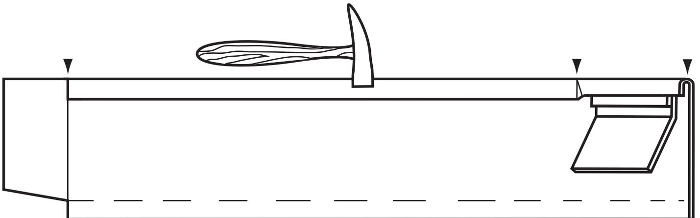
Bend the strip into a circle with the tab and the folded edge on the outside.
