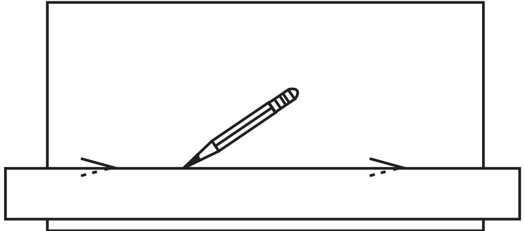
The marking gauge scratches a line parallel to the edge of the sheet. Here the gauge is used to make a line 12 mm from the edge. Hold the marking gauge 90 degrees to the edge of the sheet.
