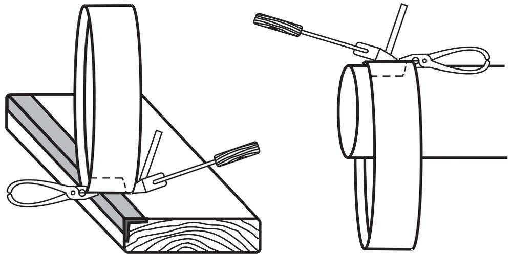
Use the marking gauge to mark 10 mm from the bottom edge. Make a small cut to the line about every 15 mm. Cut carefully to the line, not more, not less. This will help make a good joint.
