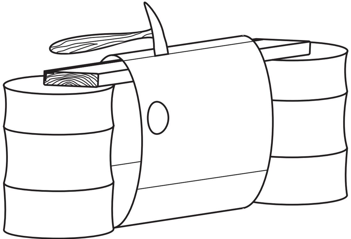
Solder the seams on one side of the sheet. The seam must be completely sealed with solder. The side with the solder will be the outside of the silo.
