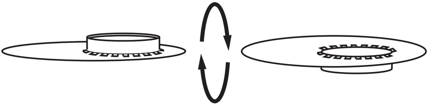
Bend some of the teeth to hold the opening in place. Go around the circle with the hammer and use the edge of the bench. Pound the teeth flat.
