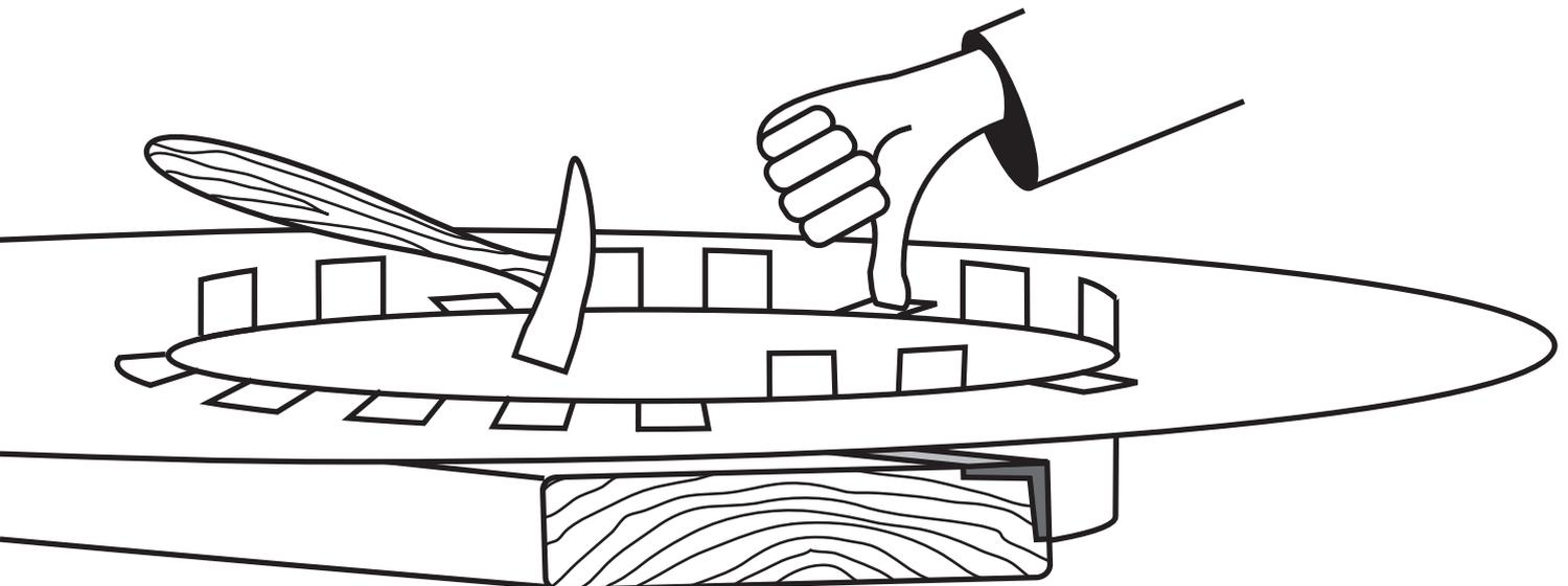
The top of the silo is now ready to be joined to the body. Use the flange method that you used to attach the bottom of the silo to the body.
