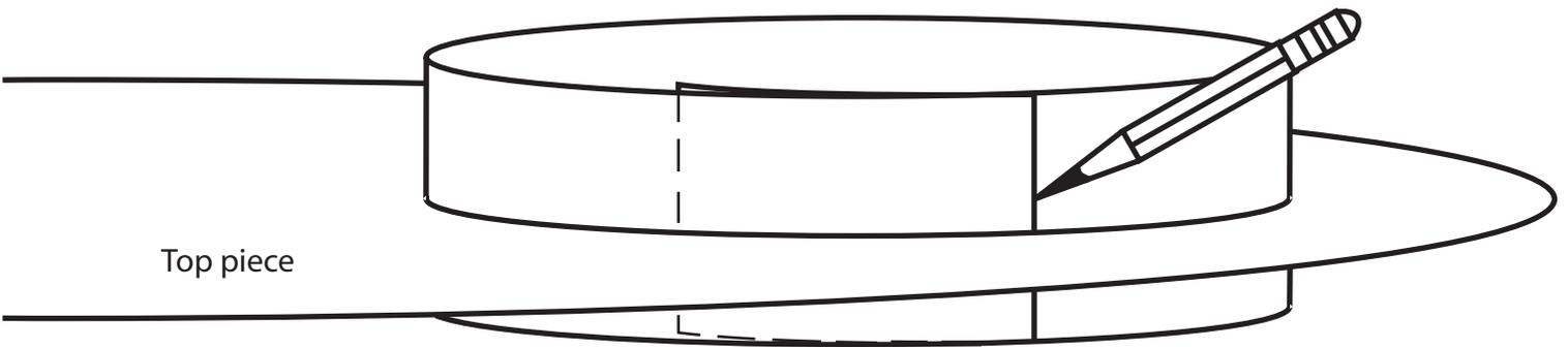
Make the strip flat again. From the mark you made, add 2 cm to make the piece longer. This 2 cm will be the tab. The tab needs relief cuts so that the edges of the strip can be folded.
