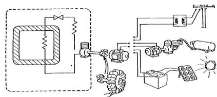
Figure 1c: Compression refrigerator
