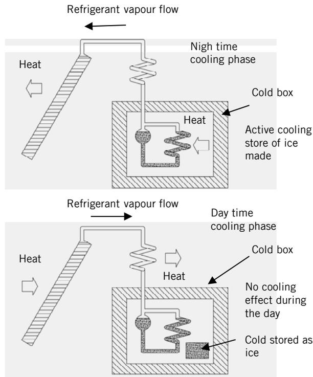
Heat phase: At high bed temperature and systems pressure, the refrigerant is driven out of the sorbent and collects in the cold box as a liquid
