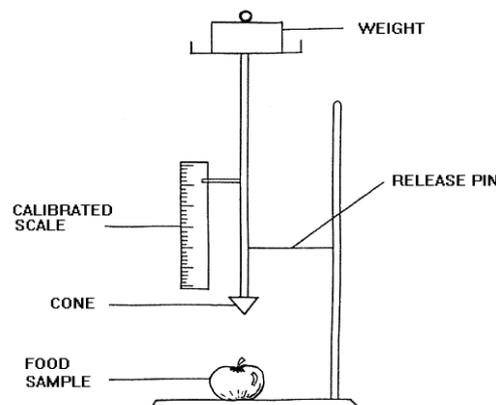
Figure 1: Fruit hardness test using a penetrometer.
