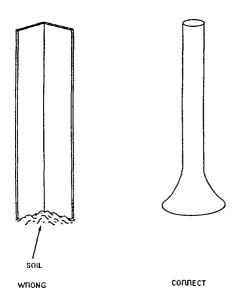
Figure 1: Support leg design to prevent soils accumulating
