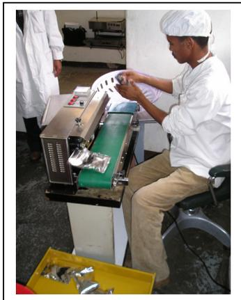
**Fig. 11.** Band sealer for plastic film
