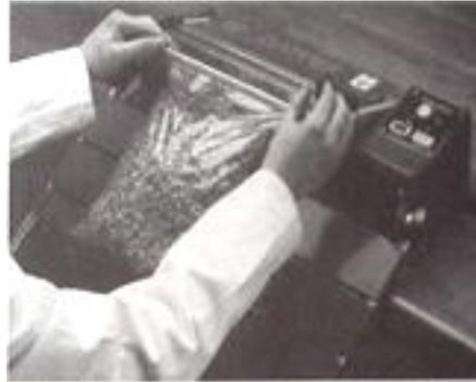
**Fig. 10.** Bar sealer for plastic film
