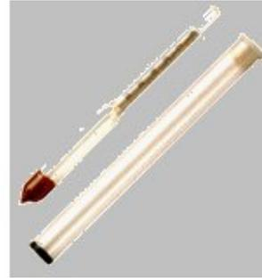
Figure 5: Salometer used to test brine strength
