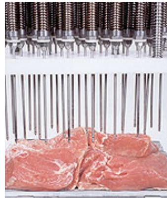
Figure 3: Brine injection needles. Photo from Cyborg Equipment Corporation
