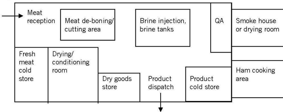
Figure 2: Layout of a meat processing room
