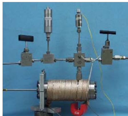
Figure 13. Photograph of solubility measurement vessel and adjacent components.
