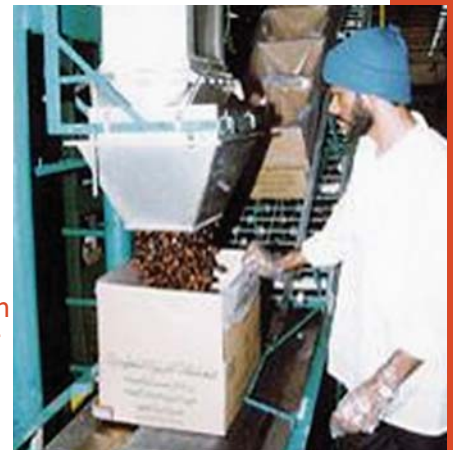
Figure 22. Bulk packing of dates into fiberboard box lined with a plastic liner (courtesy of Dr. Abdullah Alhamdan)
