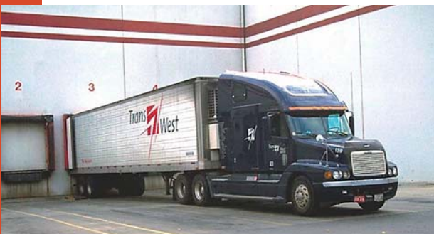
Fig. 28. Refrigerated truck being loaded from a refrigerated loading dock
