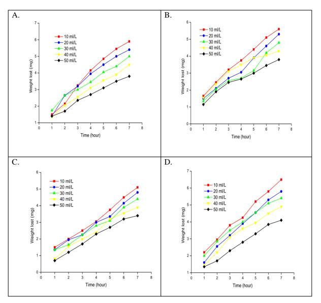
**Figure 3.** Weight loss of aluminum in different concentration of HCl media for 7 hours in the present of Nipah extract solution (A = upper frond, B = lower frond, C = inflorescence stalk, D = husk)
