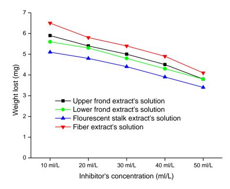
Figure 2. Overall weight loss of aluminum in different concentrations of HCl (after 7 hours)
