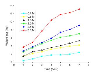
Figure 1. Weight loss of aluminum sheet in different concentrations of HCl for 7 hours
