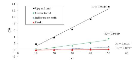
**Figure 4.** Langmuir adsorption model on Al surface of Nipah extract solution in 2.0 M HCl for 7 hours immersion period.
