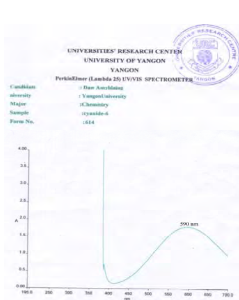
Figure 8. The absorption spectrum of hydrindantin developed from standard cyanide solution
