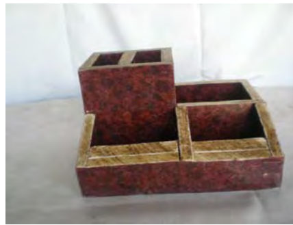
Photographs of Tissue Box and Pen Holder Made from Bagasse Based Fiberboards
