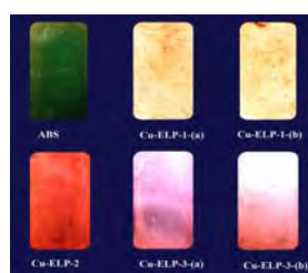
Figure 1. Three type of reducing agent on ABS plastic before and after coating of copper
