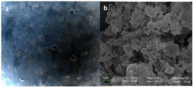
**Figure 1.** Fluorescence Microscopy (a) and Scanning Electron Microscopy (b) of *Lannea microcarpa*/NaCMC powder (LmC) produced microparticles. The images show the powder in amorphous state with well formed, small and trendy spherical microparticles with a smooth surface.
