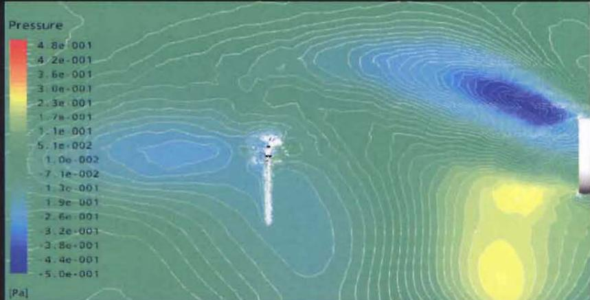
Fig. 5-6: The corresponding pressure fields of (a) and (c). The air jet is released from a  $\phi$  90-mm nozzle (on the right). Shown are the initial jet velocities.
