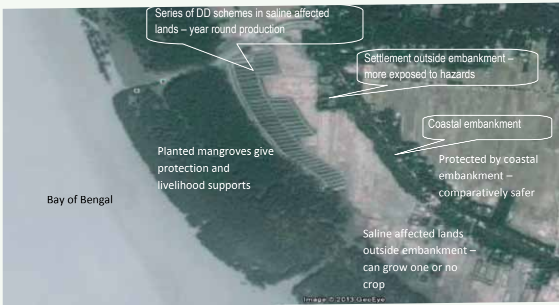
Ditch-and-dyke (DD) schemes in saline-prone lands in Noltona Union, Barguna sadar.
