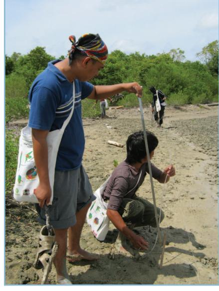
**Fig. 5.14** Using a water level to measure substrate elevations towards the landward edge of the mangrove which is rarely inundated by high tide.
