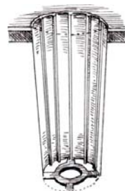
REX tray root trainers have deep longitudinal grooves to direct root growth downwards.
