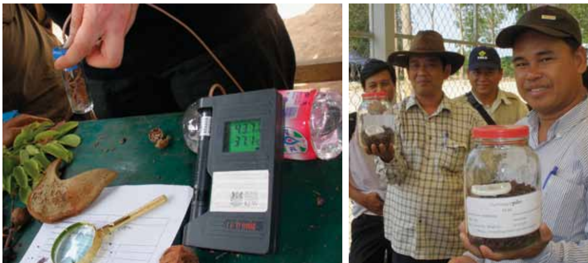
Either a sophisticated and expensive digital hygrometer (left) or simple and cheap dial hygrometers (right) can be used to assess the moisture content of seeds.
